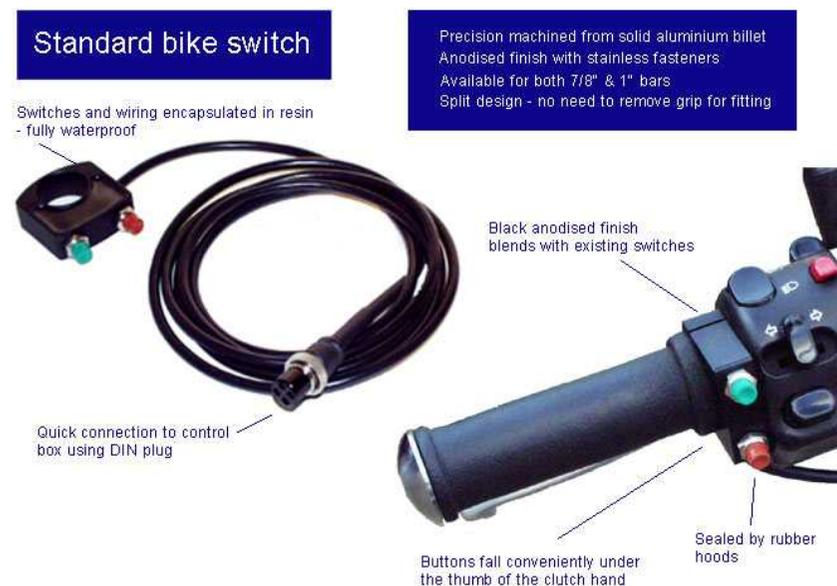
The standard on-bar switch illustrated above is normally fitted to the left-hand bar so that the buttons fall conveniently under the thumb of the clutch hand. Sometimes it is possible to move the switch cluster along the bar to accommodate the switch assembly. If not then use a sharp knife to remove a small section of the rubber grip to suit - (not possible if you have heated grips use the under-bar switch instead).
