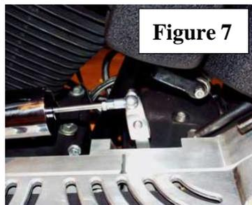
This then requires an extension piece in order to get the correct alignment and stroke from the arm which comes directly off the gearbox selector spline.
