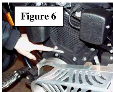
If you do not need to retain the existing linkage then it is possible to pick up on the centre bolt which runs through the centre of the 'V' between the cylinders.
